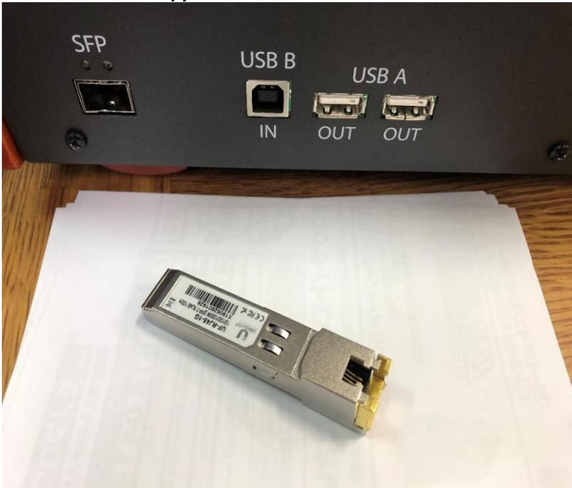
2: Insert the SFP Copper module into the SFP slot
