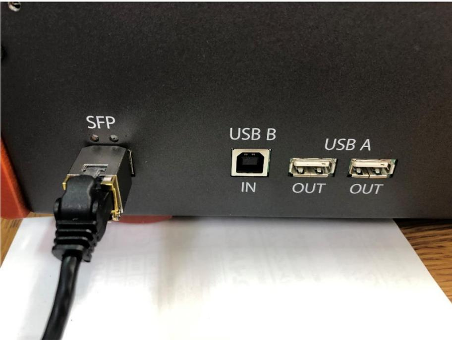
**4: Remove the SFP Copper module**
