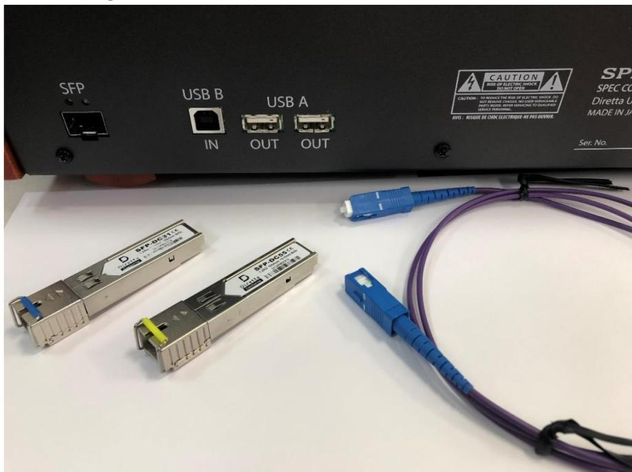
2: Insert the SFP module into the SFP slot
