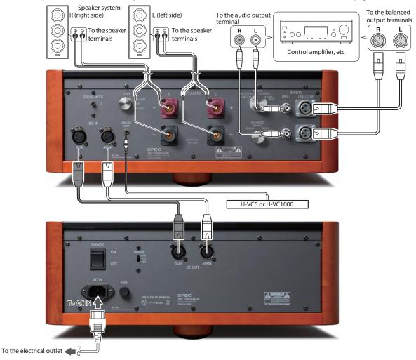
• Depending on the Control amplifier used, there may be a caution regarding simultaneously connecting RCA and XLR, so refer to the operation manual of the respective Control amplifier.
