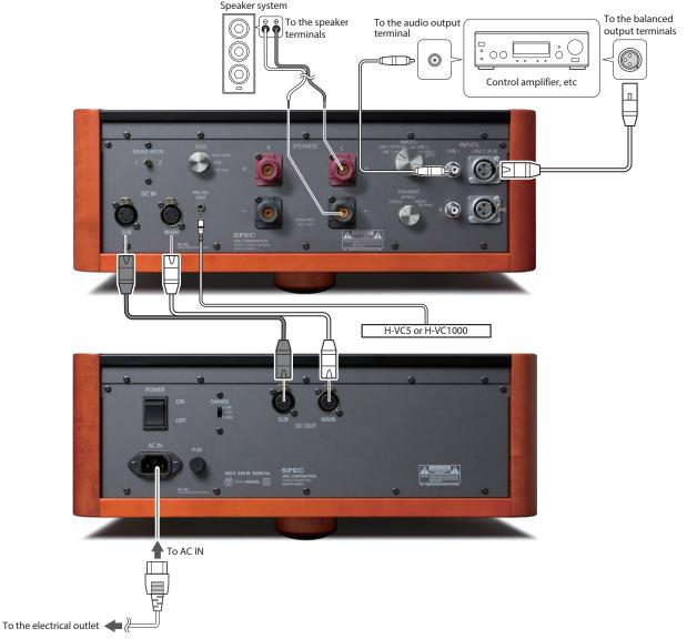
\* Depending on the control amplifier used, there may be a caution regarding simultaneously connecting RCA and XLR, so refer to the operation manual of the respective control amplifier.
