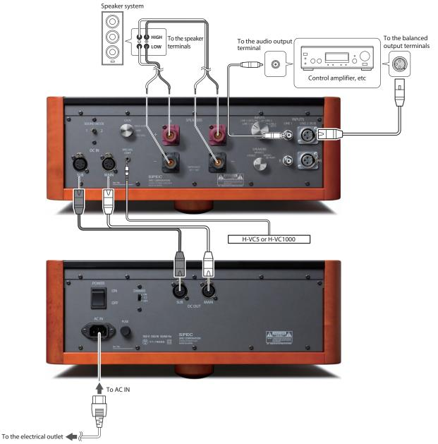
\* Depending on the control amplifier used, there may be a caution regarding simultaneously connecting RCA and XLR, so refer to the operation manual of the respective control amplifier.
