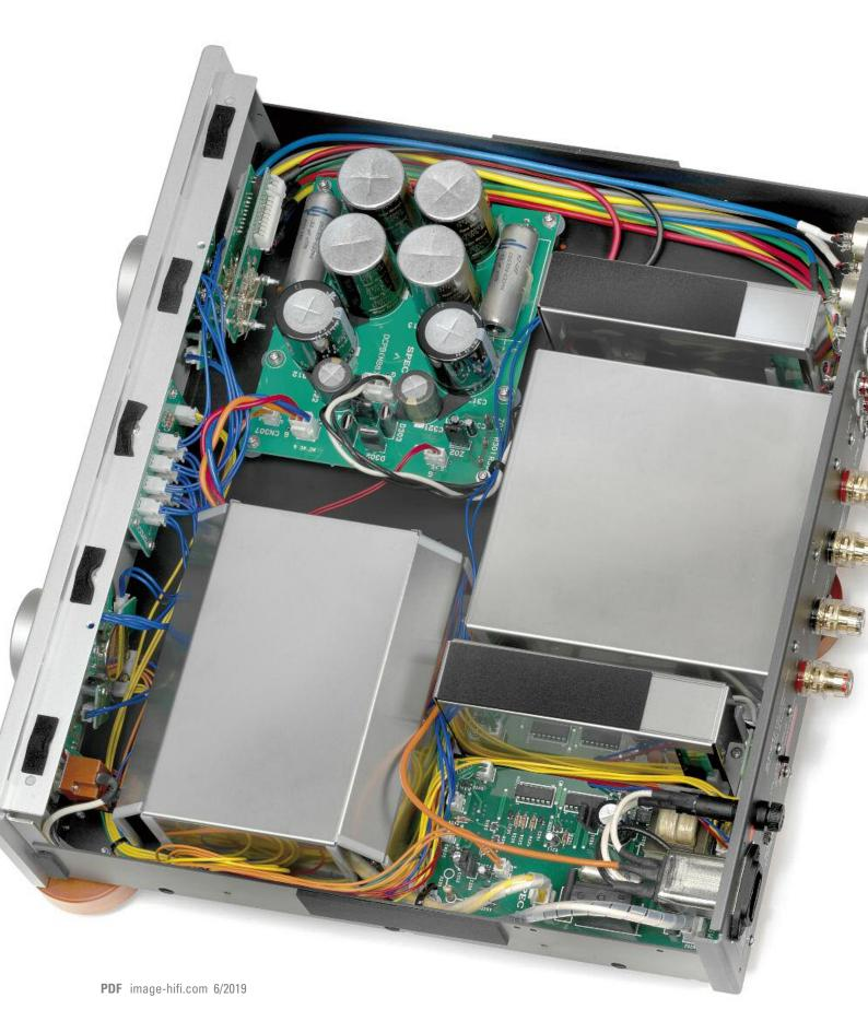
Left: Prevents electromagnetic interference: transformer section, circuit board with low-pass filter and choke circuit as well as the printed circuit boards featuring the pre and power amplifier sections are all shielded individually
