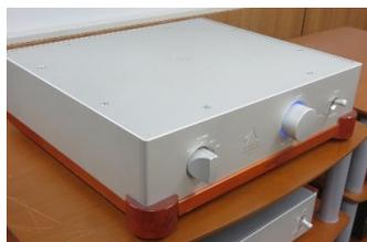
A sealed structure is possible because no holes are required for heat dissipation. Since the dust do not enter into the amplifier, the interior is kept clean for a long time. Therefore, it is also hard to break down.
